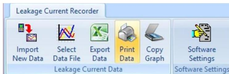
Select the *Print Data* button to print the data in a table format to the selected printer.
