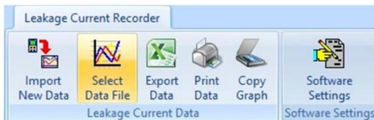
Select the *Select Data File* button and use the *File Dialog Box* to select previously imported data. The data file name consists of the Serial number of the LC-Track the data belongs to, together with date and time the data was imported. Note that the data file extension is \*.LCT. Once a file has been selected and opened the data in that file will be displayed.
