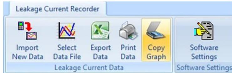
Select the *Copy Graph* button to copy the graph to the Windows clipboard, from where one can paste the graph into any windows program that supports the windows clipboard functionality (Word, Excel,...).
