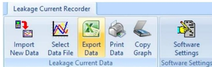
Select the *Export Data* button and use the *File Dialog Box* to specify a file and filename where the data needs to be exported to. Note that the data is exported to and Windows Excel (\*.xls) format and can be directly open using Excel.
